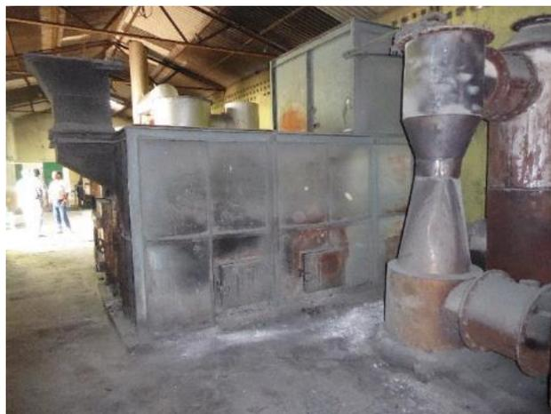
One of the facility's two incinerators, the waste is fed through the access door in the centre of the picture.
