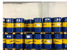
Picture 1: Packed PCB at the Treatment Plant
